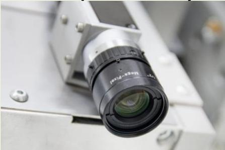
The optical camera system picks up conventional registration marks and adjusts the cutting paths position and angle where necessary to give exact marks on printed shapes.
