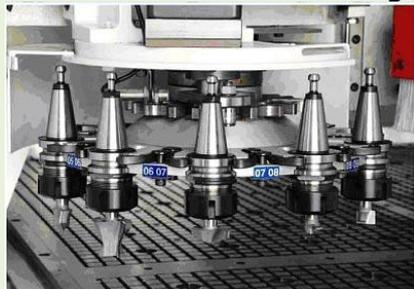
The carousel automatic tool change system gives noticeably faster tool changing which allows for production times to be decreased and therefore, production itself is increased.
