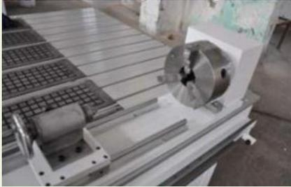
The rotary device suits cylindrical engraving and flat material carving and cutting. Items such as stair posts and columns are produced with ease with the rotary device.
