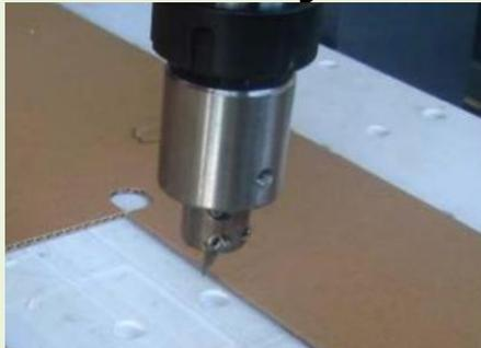
The tangential knife is a robust knife cutting tool intended for heavier, thicker and harder materials than a traditional drag knife can accommodate. A tangential knife is a cutting blade that follows the plot lines of a shape by incrementally rotating the blade to match the path.
